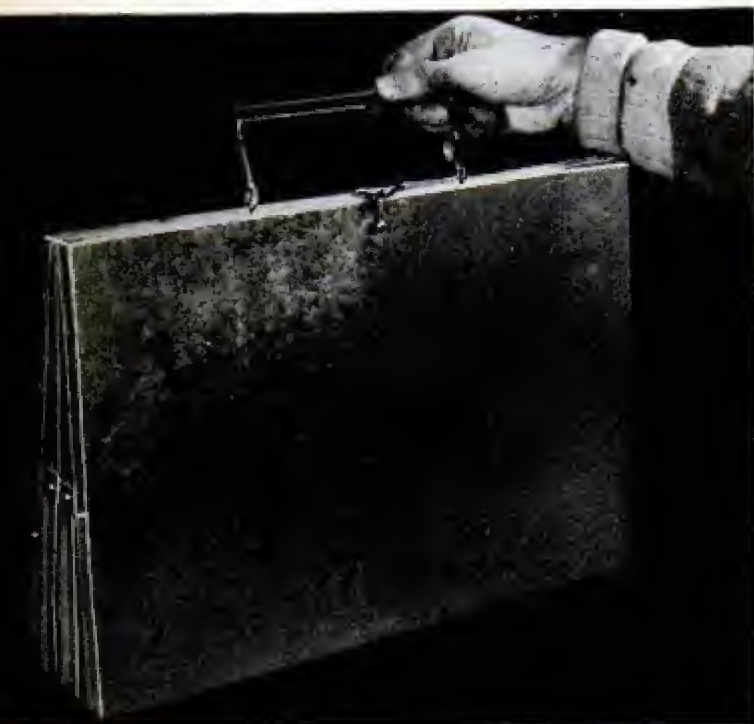
Folded, the oven resembles a neat, metal brief case. Pivoted arms fold flush with sides of oven proper
